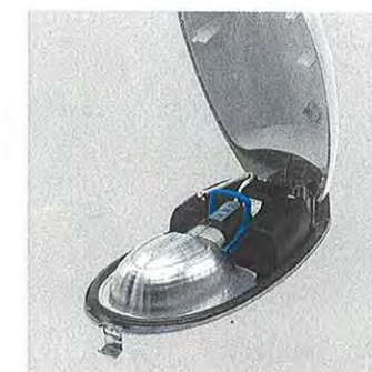
"Opti-C", where the reflector forms one unit with the bowl, and the lamp holder is attached to the reflector. This requires no internal cleaning of the optic assembly.
